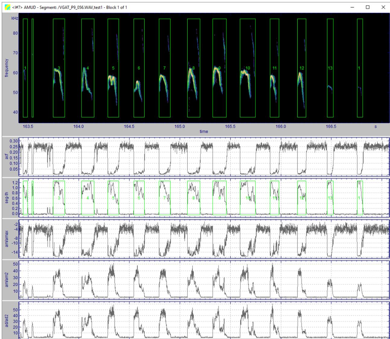
2. This picture shows a spectrogram of a very short signal part (~500ms). The automatically detected USVs are marked with red rectangles. The lower graph shows the rms-energy for the frequency bands 5kHz-40kHz and 40kHz-120kHz. This plot was created with the standard spectrogram & parameter analysis function of STx.
